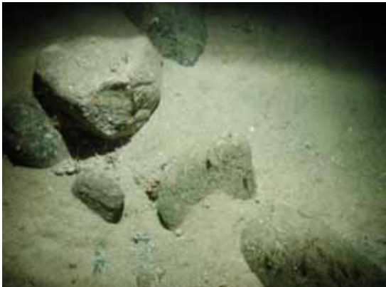
Side scan image: Ridges (waves?) of coarse and soft sediment Interpreted acoustic data: Sand covered rock and sand Location: Northern margin of Pobie Bank Still A: Coarse sand. Still B: Mixed sand and boulder.
