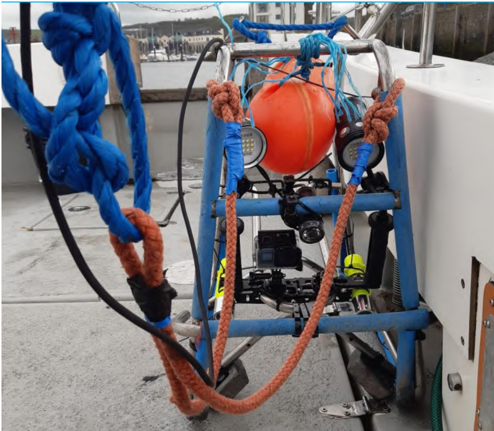
Figure 3. The camera system designed by ENVISION for benthic survey.
