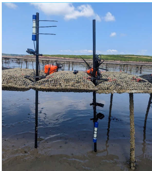
Figure 2. Example of oyster farm (test area) camera system.
