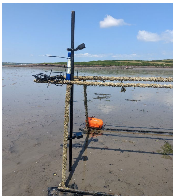
Figure 3. Example of control area underwater camera system.
